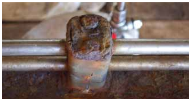
Crevice corrosion between the tube/tube trap interface.
