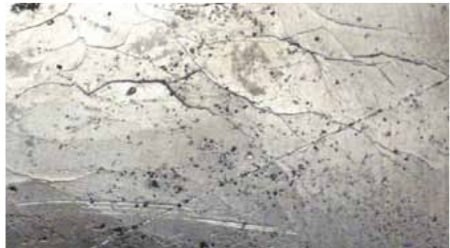
Stress Corrosion Cracking Stainless Steel in Seawater Environment
