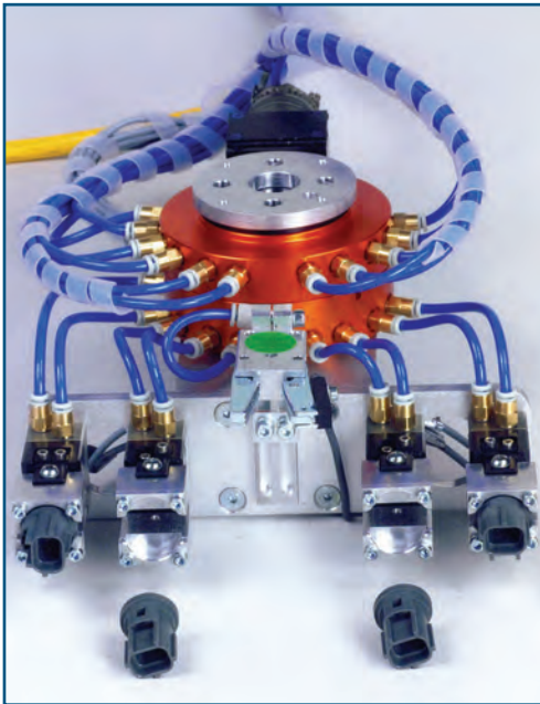
Custom EOAT for electrical plugs utilizes parallel grippers with custom manufactured jaws and a hands free quick change chuck.
