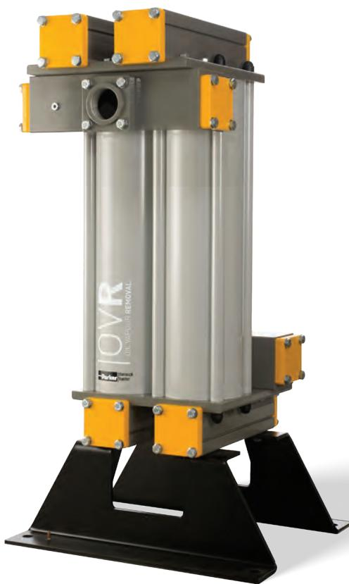
OIL-X OVR Oil Vapour Removal filters are designed to reduce oil vapour and also overcome the issues of traditional loose filled carbon towers. The loose filled beds of carbon towers offer reduced contact time due to unrestricted air channelling, meaning they are prone to movement of the carbon adsorbent during operation; resulting in degrading performance, attrition of the adsorbent material, high particulate generation and blockage of downstream filters.
