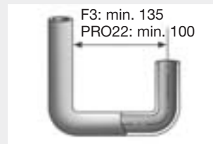
● Minimum clearance of U-shape bends
